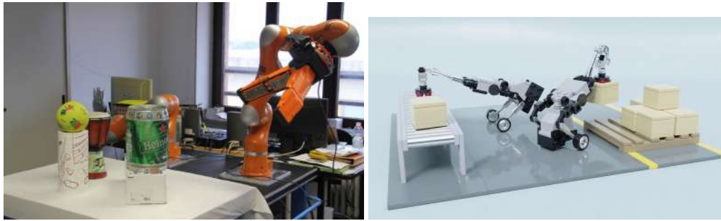
(a) The velvet finger mounted on a KUKA LWR ©2014 IEEE. Source: adapted from [82] (b) A reproduction of the Boston Dynamics Handle. Source: https://www.flickr.com/photos/87587140@N07/32549641707/
