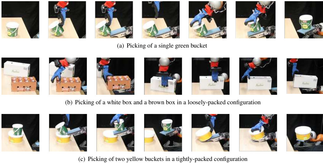
Figure 5.15: Photo sequences of the experiments addressing the three manipulation cases: single object, loosely-packed objects, and tightly-packed objects.
