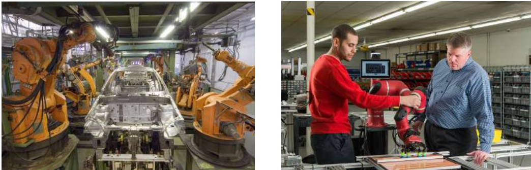
Figure 1.2: Traditional industrial automation on the left. Modern collaborative robots that can work side-by-side with humans on the right. Source: https://commons.wikimedia.org .
