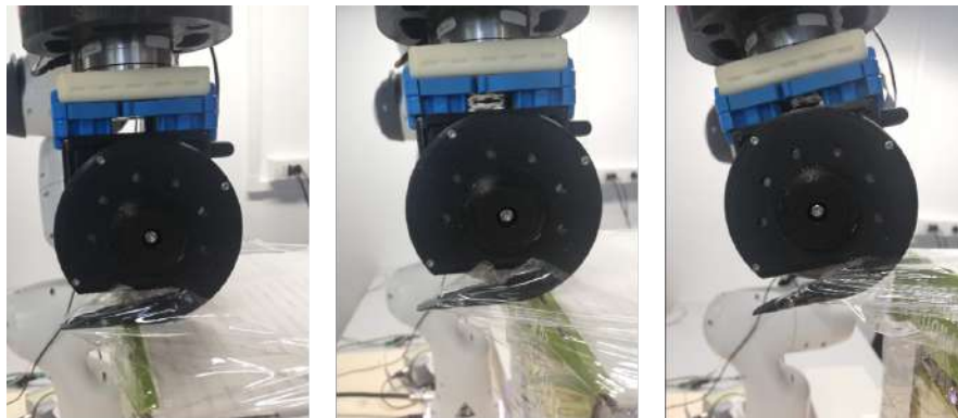
(b) The cutter rotates too late causing the rupture of the film.
