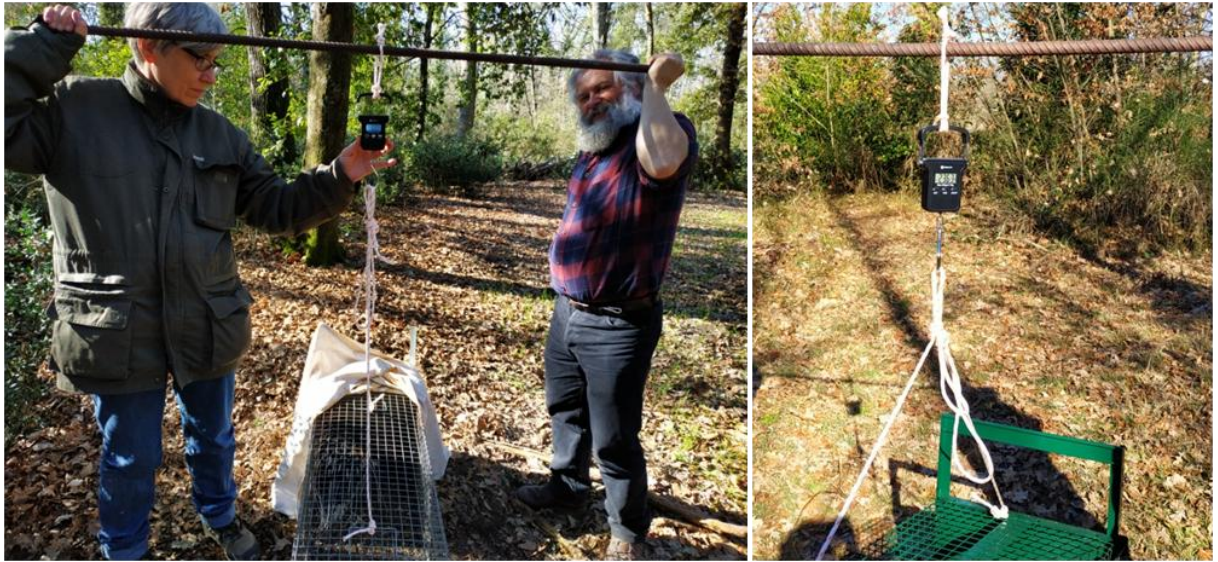
Figure 41. Weighing operation of captured porcupines. In the left two operators while raise the capture trap with the porcupine inside and in the right the detail of electronic dynamometer using for weigh the animals (Photo by Coppola and Felicioli)
