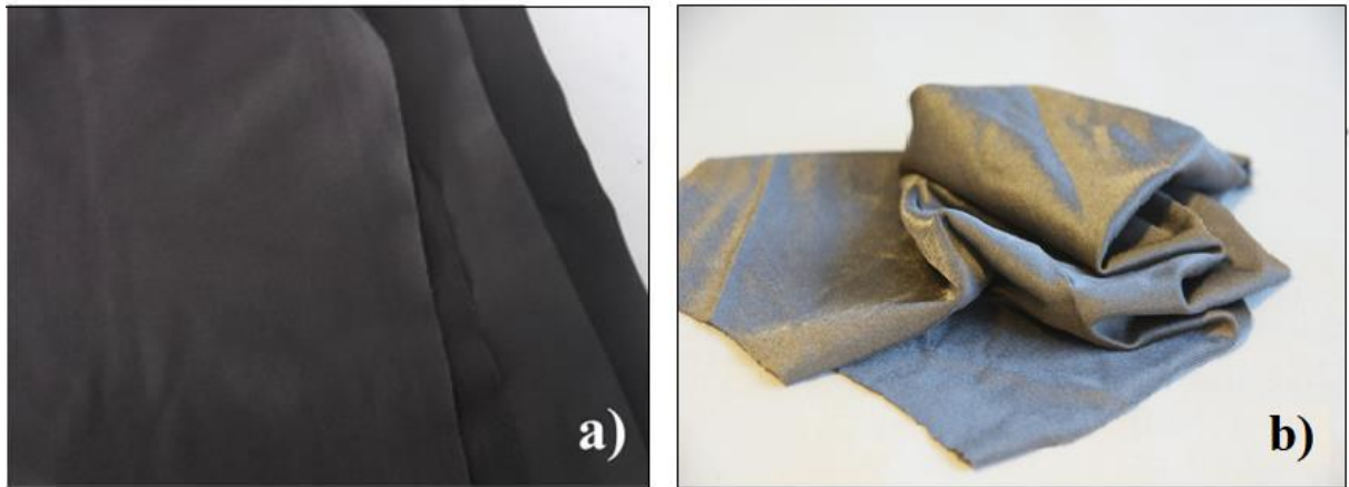
Figure 1.12 a) EeonTex™ Conductive Textiles by Eeonix Corp. [122] and b) Electrolycra by Mindsets Ltd [123].
