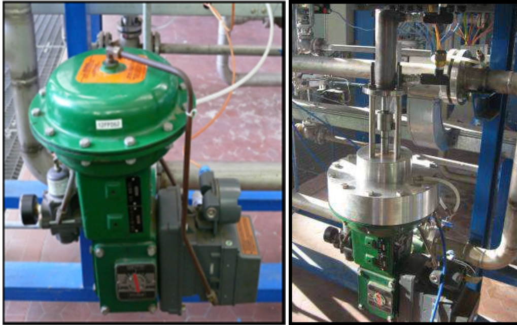
(a) Actuator, valve and positioner
