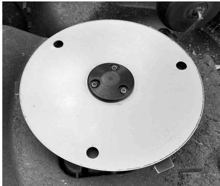
Figure 3.1. Cutting disc of the ordinary autonomous mower. Note the stainless loose disc and the pivoting cutting blades underneath.
