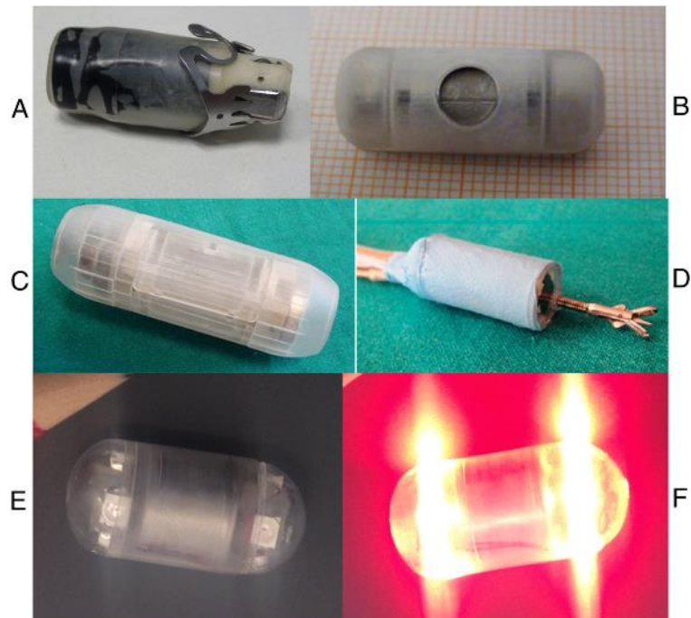
Figure 14 – a) Therapeutic wireless endoscopic capsule with an endoscopic clip for treating bleeding in the GI tract produced by Valdastrri et al.; b) Magnetic-driven biopsy capsule produced by Simi et al.; c) Therapeutic capsule for bioadhesive patch release produced by Quaglia et al.; d) Soft-tethered therapeutic capsule colonoscope developed by Valdastrri et al.; e) and f) Capsule for photodynamic therapy of Helicobacter pylori bacterium by Tortora et al.
