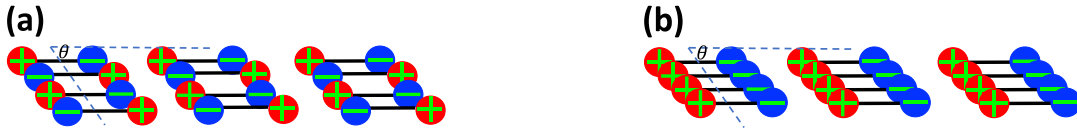
Figure C3 - extended dipole model for linear chain 2D aggregate model in J - (a) and H - (b) aggregate arrangement. Extension to the 3D model is straightforward by just vertically stacking the 2D aggregate.
