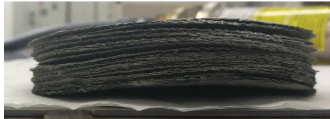
Figure 6.7 – Delaminated preform after MW-CVI runs
