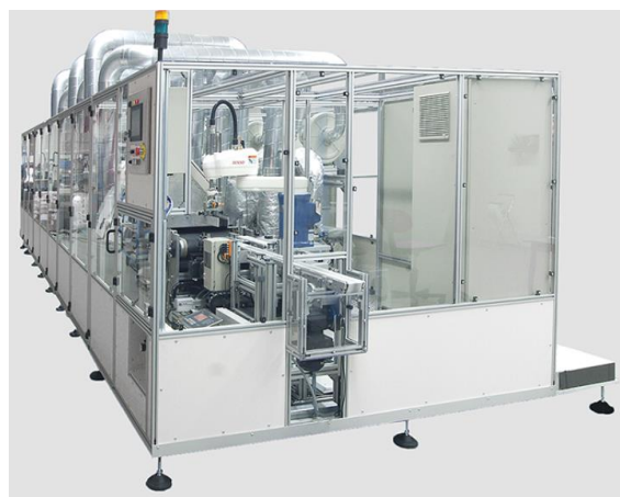
Figure 1.7 - Microwave hybrid continuous dryer for fast and homogeneous drying of technical ceramics developed by Fricke und Mallah Microwave Technology [66]
