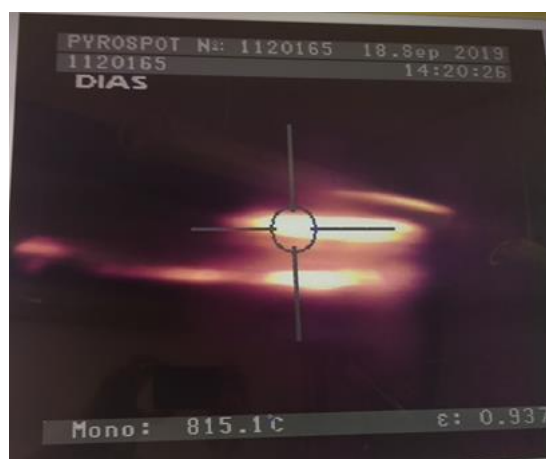
Figure 6.3 - Thermo-camera image at the infiltration temperature
