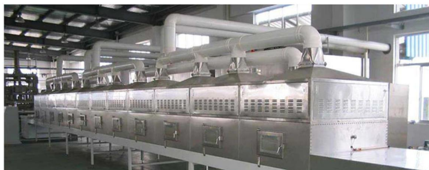
Figure 1.5 - Industrial Microwave Tunnel Conveyor Machine developed by Max Industrial Microwave [63]
