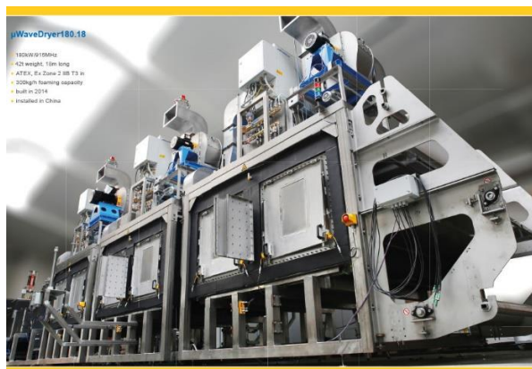
Figure 1.6 – Microwave drying system developed by Püschner Microwave Power Systems [65]
