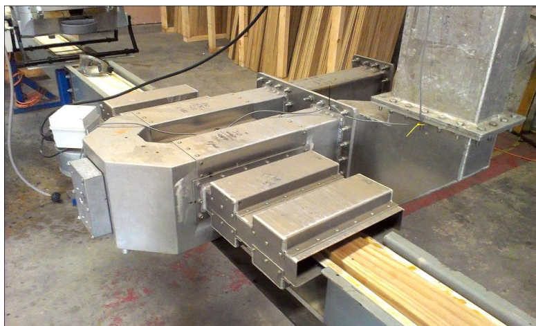
Figure 3.12 – Image of a 922 MHz "meander line" travelling wave applicator [51]
