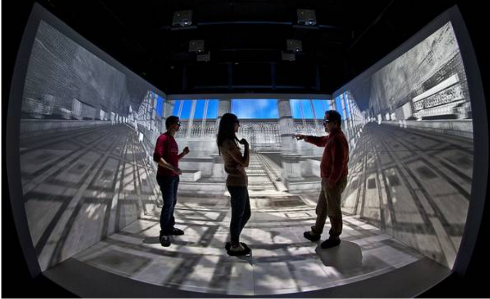
Figure 4.4: The 6-nodes and 18-projectors CAVE setup used to run performances tests.
