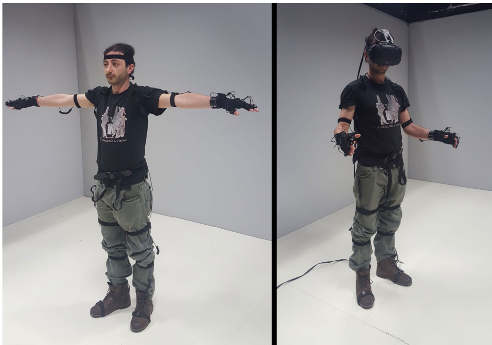
Figure 5.5: A user wearing the MOCAP suit. On the left the user is performing the suit's calibration procedure. On the right the user is interacting with the VE.
