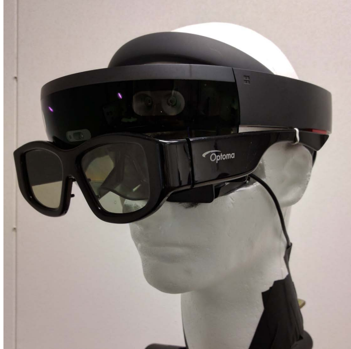
Figure 6.3: Microsoft HoloLens headset with active shutter glasses. Styrofoam head contains a camera used to capture actual footage of the see-through display.
