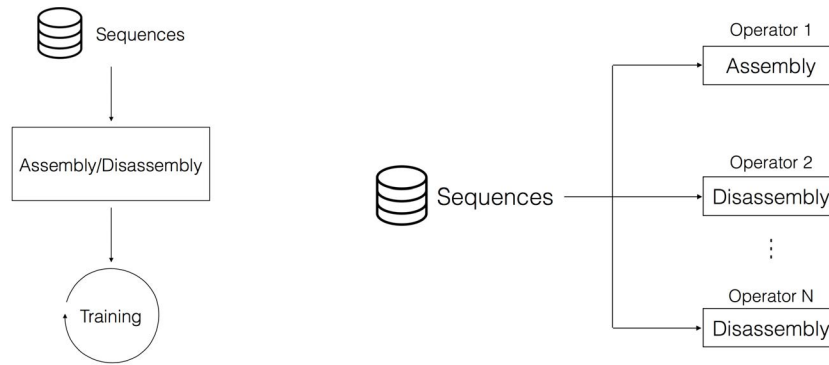
Figure 7.3: The training system flow chart. Different operators can use the same sequences to perform different tasks on the same machine.
