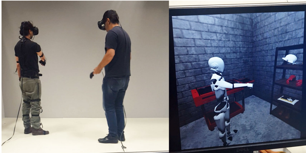
Figure 5.8: Two users sharing the same virtual space. The user on the left is wearing a MOCAP suit. The monitor shows what the user on the right is seeing.
