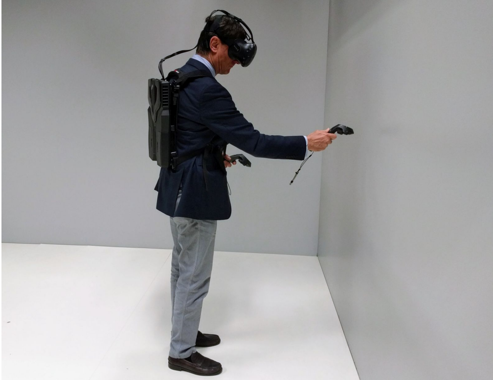
Figure 5.6: The untethered VR system exploiting a back-pack workstation.
