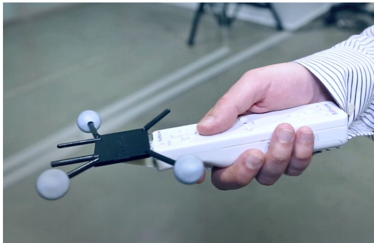
Figure 5.3: The hand controller: a Wii controller with an Optitrack's constellation mounted on top.
