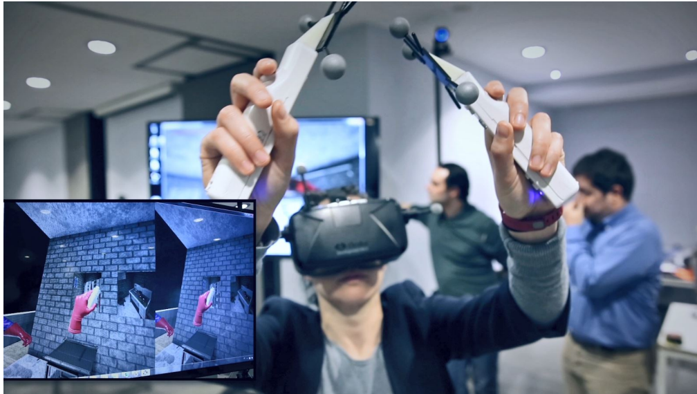
Figure 5.1: A user experiencing the immersive VR training simulator. The user physically grabbing two controllers can see his hand replicated inside the VE.
