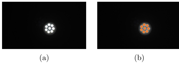
Figure 4.8: RoI-detection algorithm results by using Otsu's method thresholding: a)Original picture; b) Intensity-based detection of the light source using Otsu's method.
