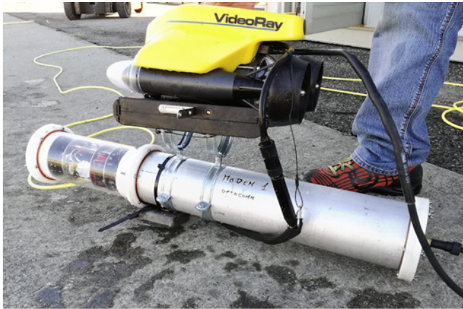
Figure 5.23: The UOWC modem equipped under the ROV for mobile transmission.
