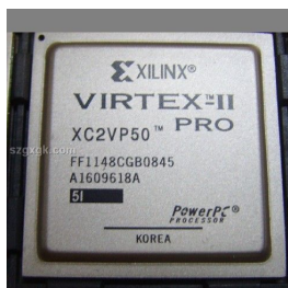
Figure 1.1: The NetFPGA main core: a Xilinx Virtex II Pro FPGA.
