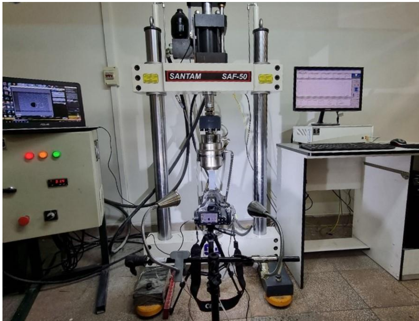
Fig. 5-3. Experimental setup employed to conduct the static and fatigue tests.
