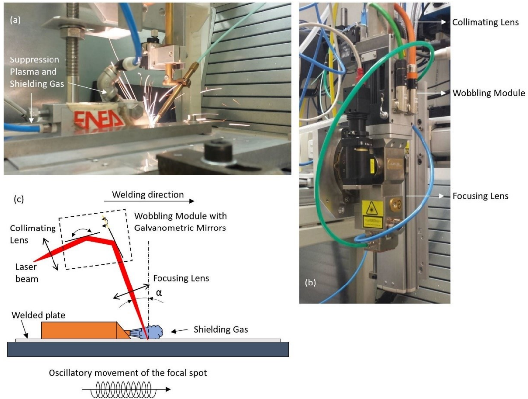
Figure 16. (a) Welding set-up; (b) welding head; (c) working principle diagram.
