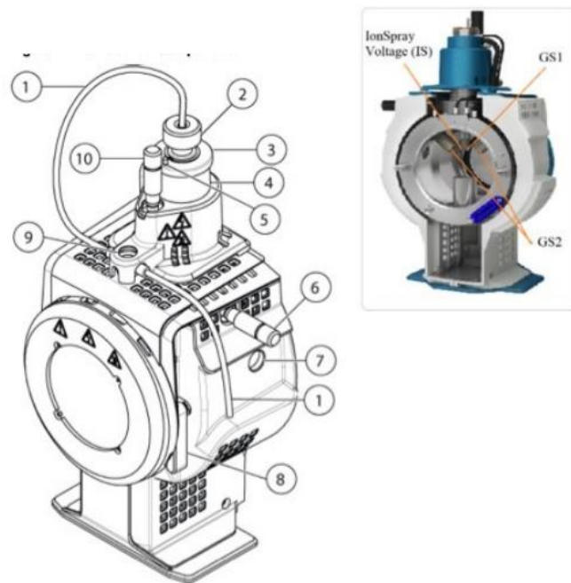
Fig.23- Ion Source Component-Item n. 1 Sample tubing, n.2 Electrode adjustment nut, n.3 Retaining ring, n.4 Probe tower,n.5 Corona discharge needle adjustment screw, n.6 Micrometer used to position the probe in the horizontal axis for ion source sensitivity adjustments, n.7 Window port, n.8 One of two source latches that secure the ion source to the mass spectrometer, n. 9 Grounding union.It is not visible below the ion source cover, n.10 Micrometer used to position the probe on the vertical axis for ion source sensitivity adjustments
