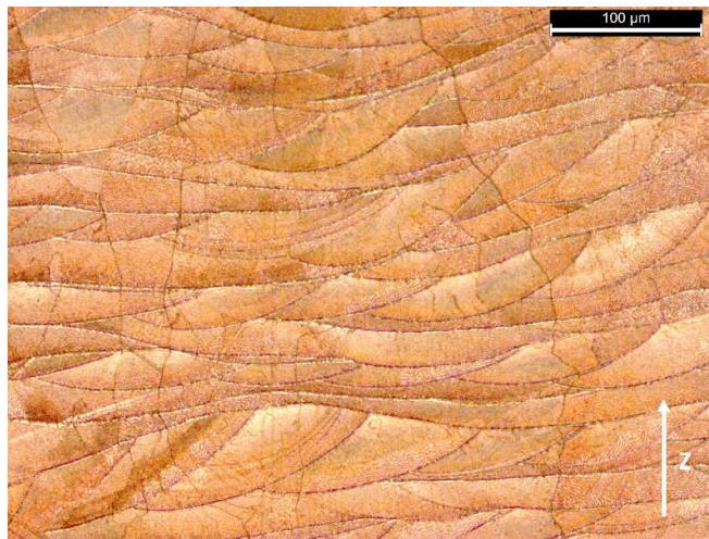
Figure 74. Microstructure of the sample 8 of the batch 2 produced by Printgreen machine (OM 200X).
