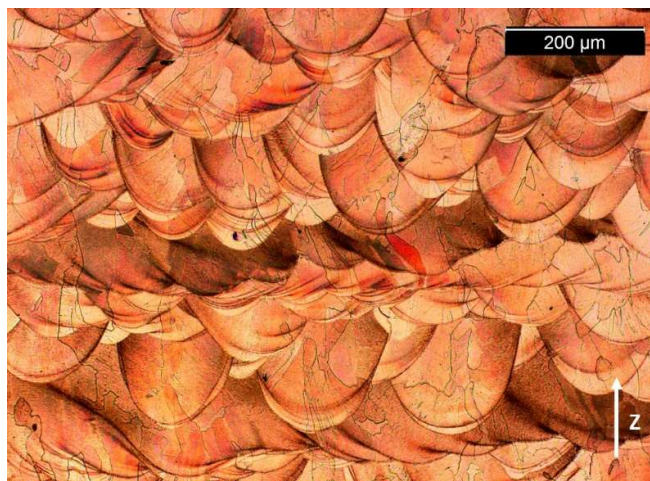
Figure 65. Microstructure of the sample 1 of the batch 2 produced by Printsharp machine (OM 100X).
