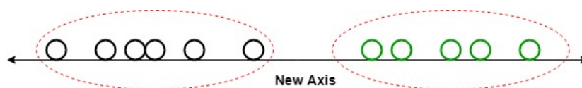
Fig. 2.22 Linear Discriminant Analysis (LDA) is used which reduces the 2D graph into a 1D graph to maximize the separability between the two classes [10].
