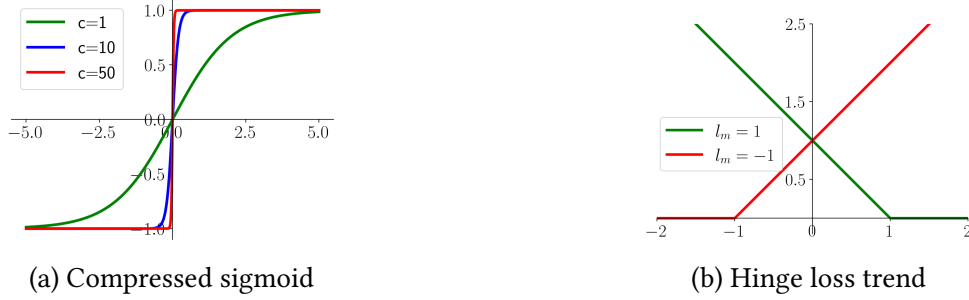
Figure 6.4: (a) Increasing c in the MSE compressed sigmoid transforms it into a Heaviside step function: the loss is zero when the output score has the correct sign. (b) Hinge loss trend for positive ( l_m = 1 ) and negative ( l_m = -1 ) pairs ( \delta = 1 ).
