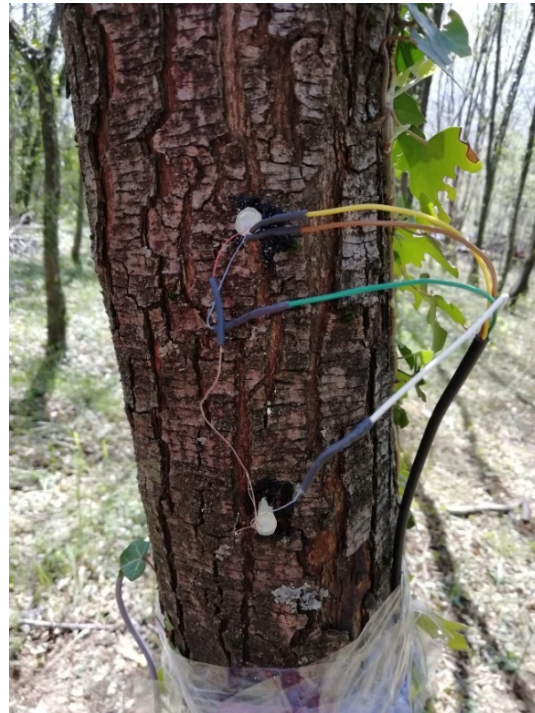
Figure 3: Sapflow sensors installed on white hornbeam (Carlino) and hop hornbeam (Caltrano). The sensors consist of 2 probes that are inserted into the trunk at a distance of about 10 cm from each other. The upper probe is heated and when the upward flow is consistent, it is cooled. In this way the temperature difference provides information on the intensity of the flow.
