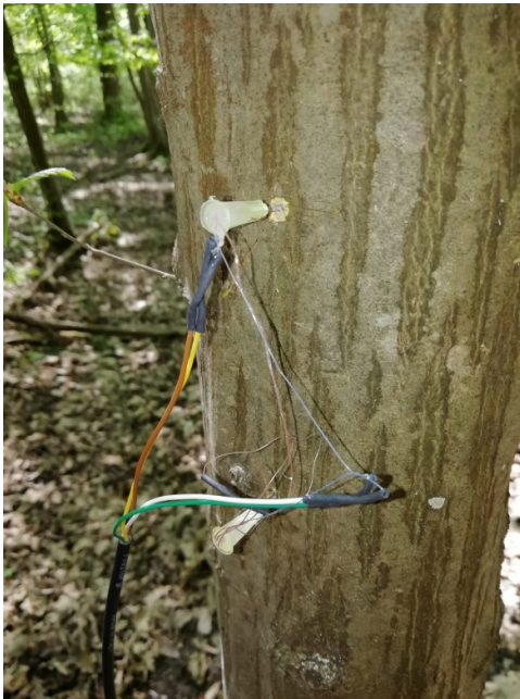
Figure 2: dendrometer installed on a tree. The potentiometer is fixed with two screws that sink into the deepest part of the trunk (not subject to movements), while the tip grazes the bark, and is pushed back and forth by the growth of the plant's radius, as well as from swelling and shrinkage due to daily cycles of hydration and dehydration
