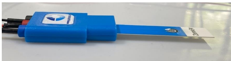
Figure 4.20: Image of SPE with immobilized yeast cells.
