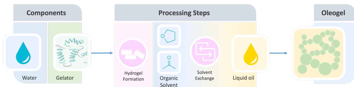
Figure 8. Schematic representation of the solvent exchange template-based oleogel.
