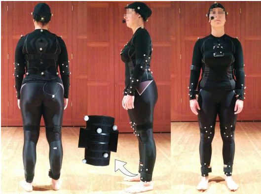
Figure 5.3: Markers and rigid bodies placed on the dancer's body. A rigid body is a rigid plate on which several markers are attached. This configuration allows us to extract not only the position but also the rotation of body joints. In the figure, a rigid body is highlighted.
