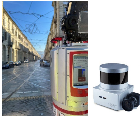
Figure 21: Examples of a Terrestrial Laser Scanning data acquisition (on the left) and a handheld mobile Laser Scanning System (on the right).
