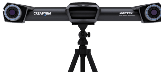
Figure 16: Example of a triangulation-based laser scanner.
