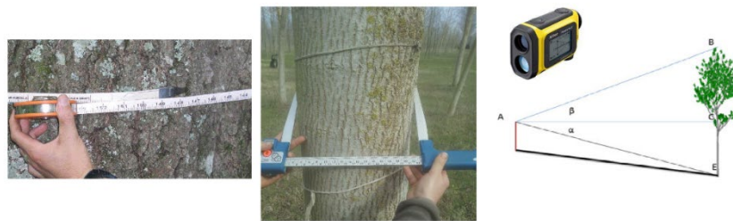
Figure 9: Examples of diameter tape (on the left), dendrometric caliper (in the middle) and hypsometer (on the right) and their functioning.
