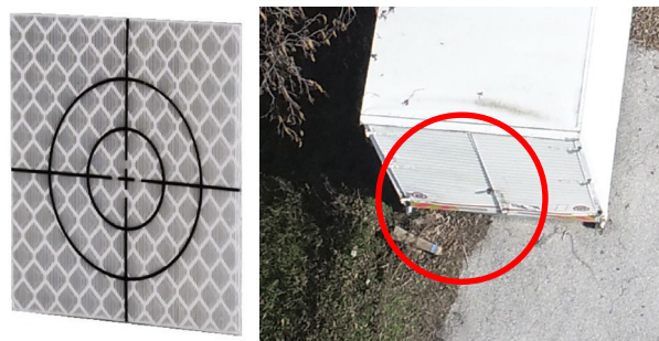
Figure 27: Examples of retroreflective targets (on the left) and edges of regular human-made objects (on the right, in the red circle) to be distinctively detected for the alignment procedure.
