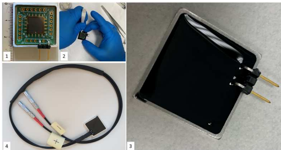
Figure 4.34 Steps of the SiC coating process, from 1 to 4 in chronological order. See text for details. The "-" label indicates the wire connected to the anode of the diode, while the "+" is connected to the cathode.
