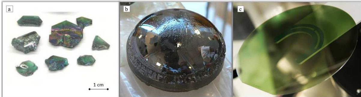
Figure 3.2 Silicon carbide in various forms. a) SiC platelets obtained in the Acheson process [239]. b) A SiC single crystal ingot synthesized via the sublimation method [300]. c) SiC wafer (200 mm) ready for subsequent processing [301].
