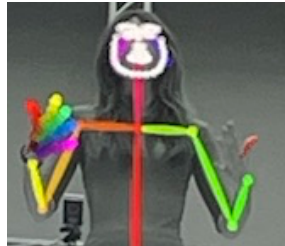
Figure 22. Failure of the use of the OpenPose system in capturing finger key points (CC BY 4.0).
