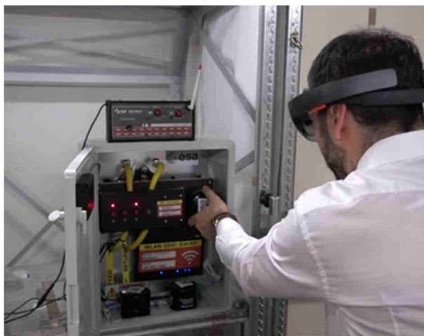
Figure 2.10 Operator using EdcAR with Microsoft HoloLens ® at work on Columbus mock-up (credit: ESA)
