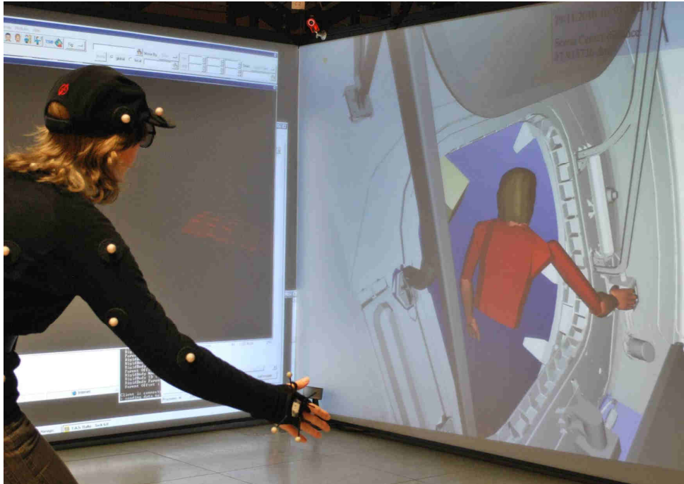
Figure 2.9 User with motion-capture sensors and the JACK Live™ mannequin virtual replica while assessing the ISS Columbus module hatch accessibility (credit: TAS-I)
