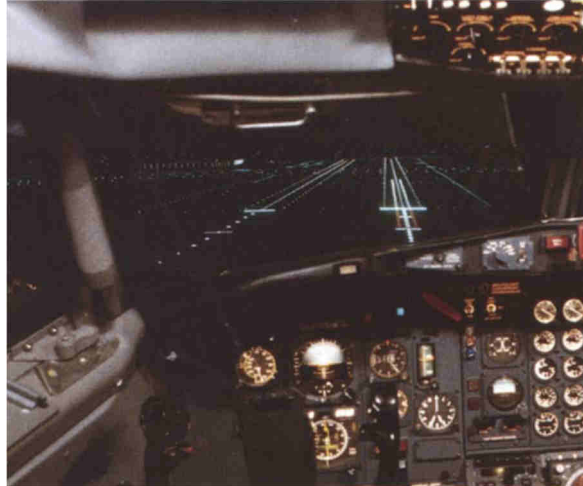
Figure 2.4 View through the cockpit of a 727 simulator at NASA Ames Research Center (ARC) which is used for human factors research. A simulated night flying environment is visible out the forward cockpit window [87] (credit: NASA)
