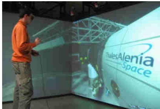
Figure 4.15 User in the Mechdyne CAVE™ while interacting with a virtual scene created using VERITAS (credit: TAS-I)
