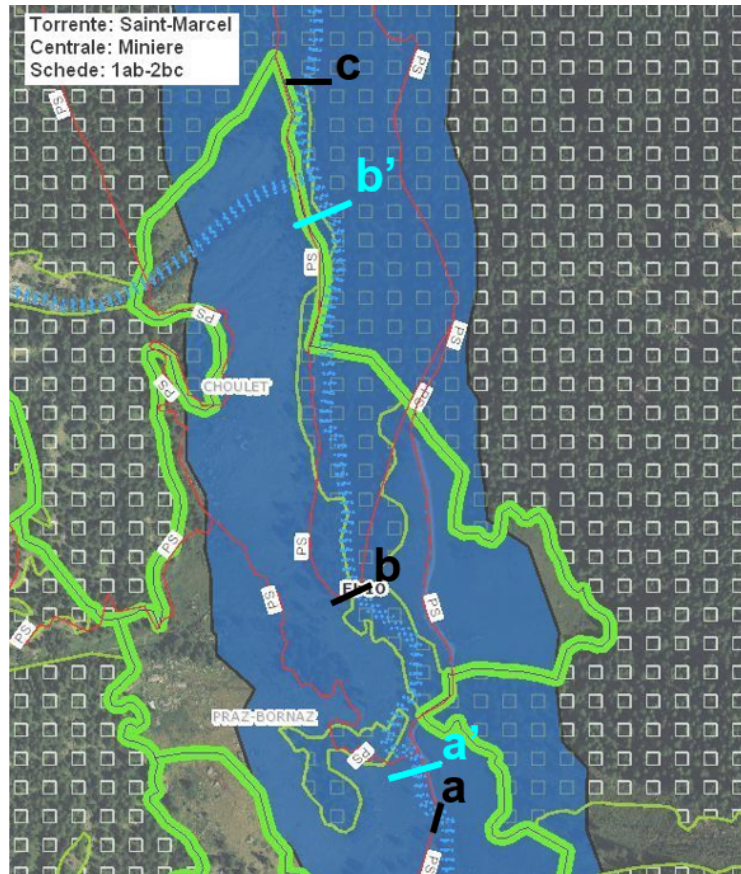
Fig. 4.3 First two subsections ( ab and bc ) into which the bypassed stretch on the Saint-Marcel torrent (case study 4) has been divided. Due to the presence of an agricultural withdrawal in b' , the hydropower producer releases the discharge required by the license in a and, from May to the beginning of October, an additional water amount in a' , which is withdrawn by the agricultural diversion in b'
