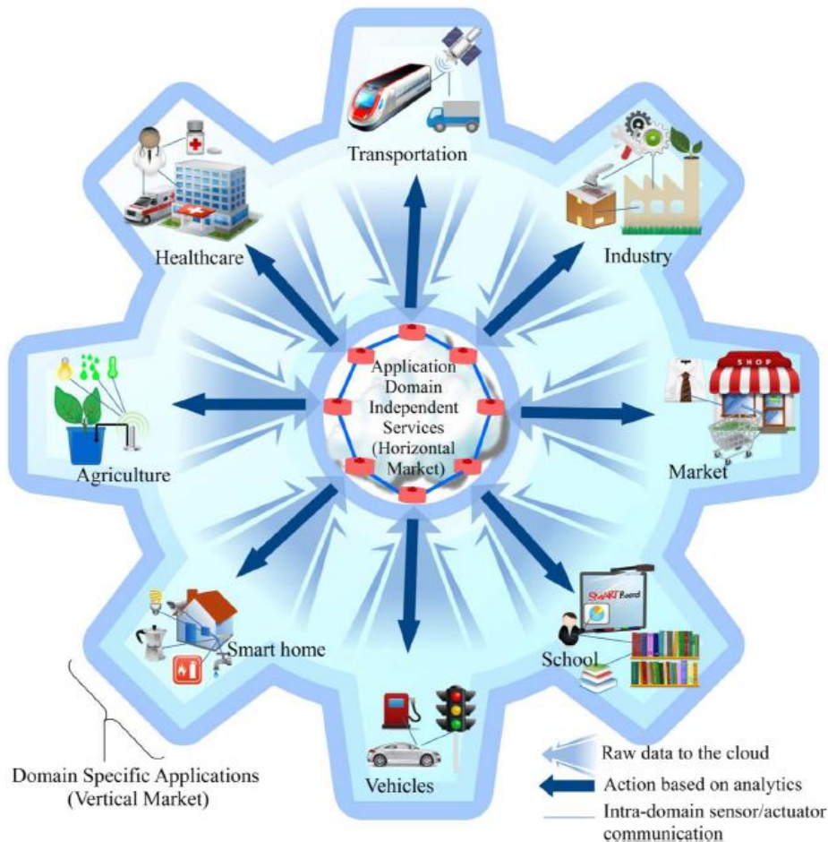
Fig. 1.1 Vertical markets : smart things with their supposed functions constitute domain specific applications. Horizontal markets : application domain independent services with ubiquitous computing and analytical services [1].
