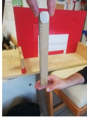
(a) Ruler Test set-up
