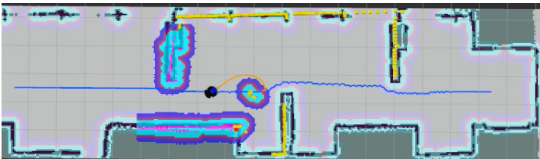
Fig. 3.8 Test Case 3: OSGP algorithm reaction to generic obstacle detection.
