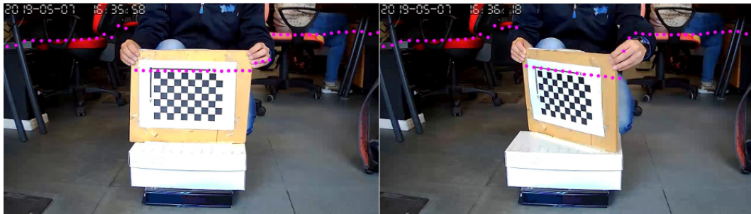
Fig. 6.3 Laser points projected in the image plane.
