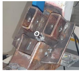
Figure 6.6. Testing frame: a) Load and constrain condition (dimensions are expressed in mm); b) test set-up; c) detail of the hinge area; the screw reproduces the end of the pedal stroke.
