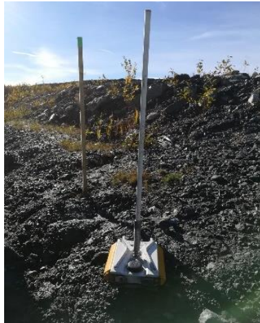
Figure 3.9: A planted 10-Hz geophone connected to a wireless station, belonging to the irregular grid of receivers of the 2018 Siilinjärvi seismic survey.
