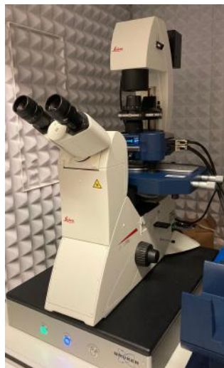
Figure 3.6 – JPK NanoWizard IV AFM (Bruker)
