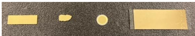
Figure 3.1 – Substrates employed in this thesis. From left to right, substrates for experiments: (1) SE/XPS: Au (250 nm) on borosilicate glass slides (with a Cr primer layer), RMS ( 2 \mu\text{m}^2 )=1.7 nm; (2) AFM: Au (100-200 nm) on silicon wafer, RMS ( 2 \mu\text{m}^2 )=0.3 nm; (3) QCM-D: Au on quartz sensor, RMS ( 2 \mu\text{m}^2 )=1.1 nm; (4) SPEE: Au (50 nm) on borosilicate glass slides (with a Ti primer layer), RMS ( 2 \mu\text{m}^2 )=1.5 nm.
