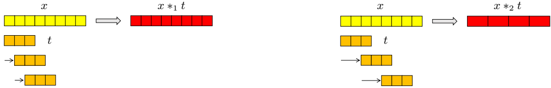
(a) Discrete convolution with stride s = 1 between an input vector x \in \mathbb{R}^8 (in yellow) and a filter t \in \mathbb{R}^3 (in orange), which gives as output a vector x *_1 t \in \mathbb{R}^8 (in red). The input and output sizes are the same.
