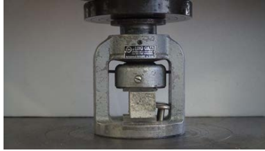
Figure 5.4 Photo of the compressive test apparatus and specimen
