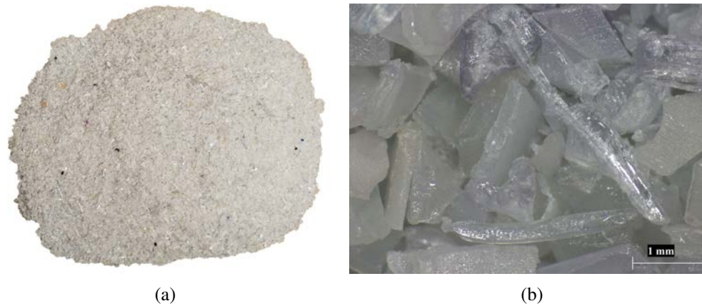
Figure 5.1 Recycled PET aggregate (a) and micro-photo (b)
