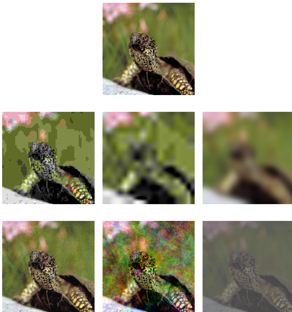
Figure 2.11: An original image from CSIQ and its most distorted versions for JPEG, JPEG200, blur, white noise, F noise and contrast artifacts respectively.
