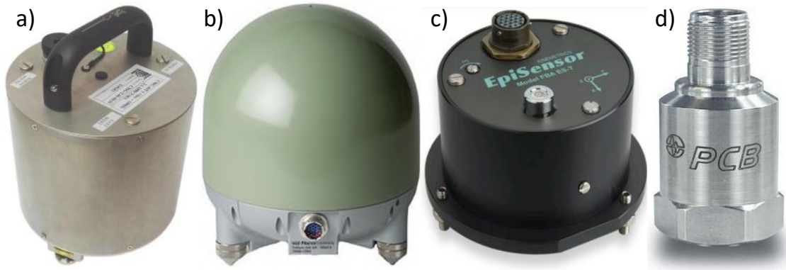
Figure 3.8: Seismic sensors used in Virgo: a) Güralp CMG 40-T seismometer; b) Nanometrics Trillium 240 seismometer; c) Kinometrics EpiSensor FBA ES-T accelerometer; d) ICP accelerometer 393B12 by PCB Piezotronics (MTS Systems Corporation).
