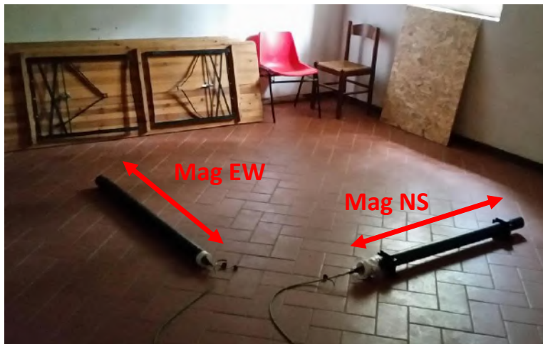
Figure 2.4: A photo of the Villa Cristina scout house interiors, where we deployed the magnetometers for a 2 days measurement of the Schumann resonances.
