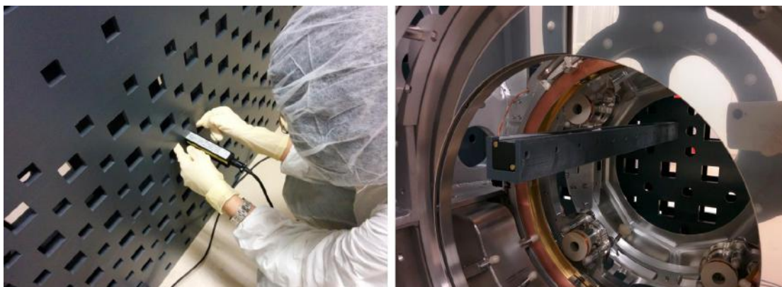
Figure 2.27: On the left is a focus on the placement of the magnetic probe inside the PVC frame. In addition (on the right), a probe-holder rod can make spot measurements along a line inside the volume of the payload.
