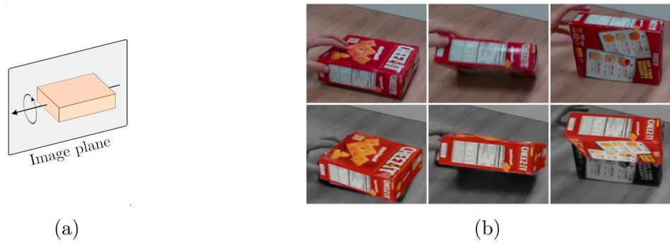
Figure 5.8 (a) Example of out-of-plane object rotation. (b) Top: input images. Bottom: example of imprecise estimates in presence of out-of-plane object rotations.
