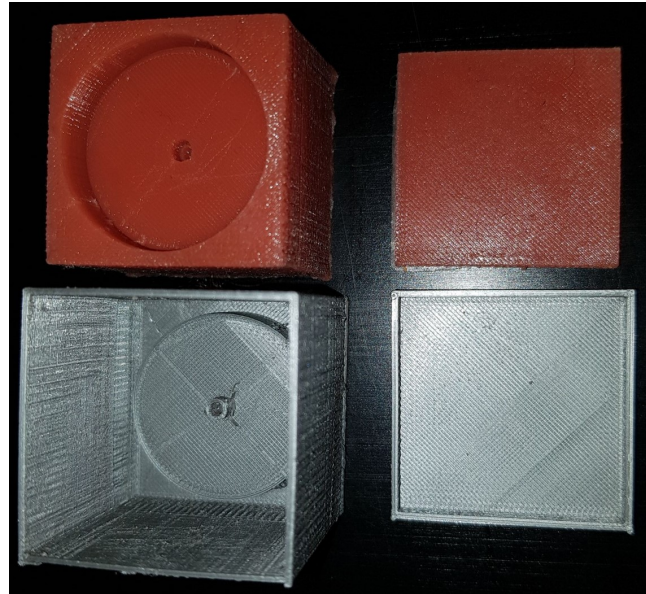
FIGURE 3.5: Molds and respective molded parts to build the SCM. 3D printed molds and the molded silicone.
