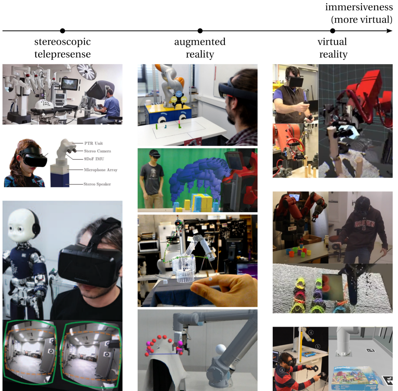
Figure 1.2: Examples of existing immersive teleoperation setups from least to most virtual, columns left to right: stereoscopic telepresence [23, 24, 25], augmented reality based robot teleoperation [26, 27, 28, 29], virtual reality based robot teleoperation [30, 4, 3].
