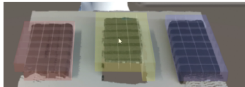
Predicted materials as colour-coded OctoMap overlay
