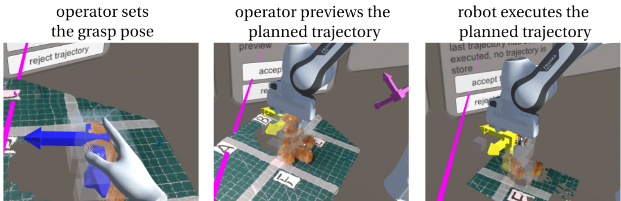
Figure 2.8: Supervised control mode: move-to-grasp.
