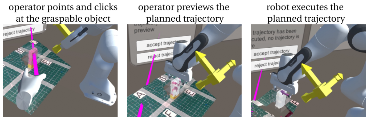
Figure 2.9: Supervised control mode: point-and-click grasping
