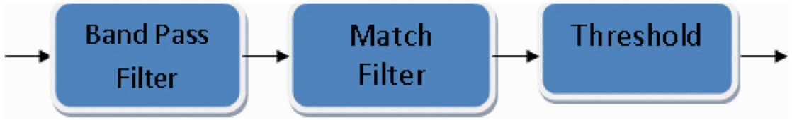
Figure 2.7: Matched filter detection block diagram
