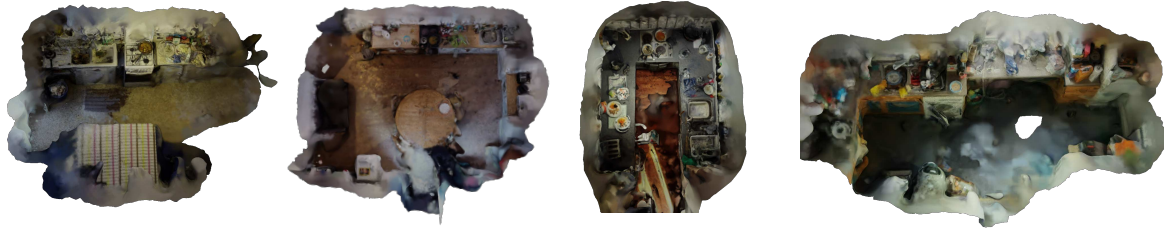
Fig. 6.2 3D reconstruction of the scenes. Example of 3D meshes of 4 different environments using Poisson surface reconstruction.
