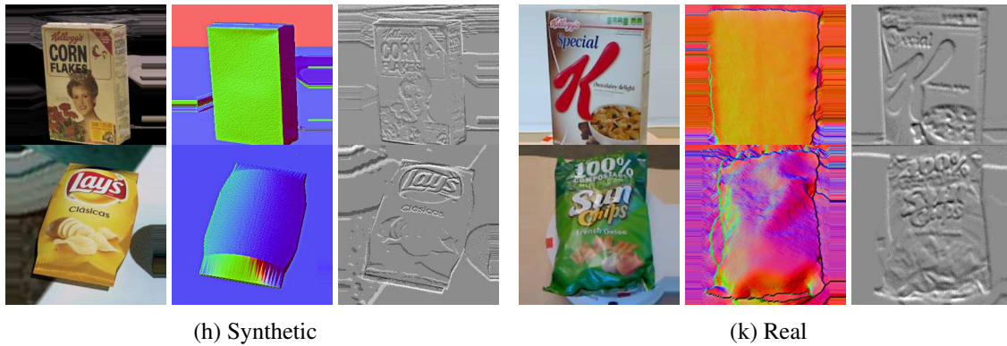
Fig. 5.10 N-ROD examples. Synthetic (left) and real (right) samples from the N-ROD dataset. Depth images are coloured with surface normal encoding and event sequences are represented using voxelgrid (Zhu et al., 2019a).
