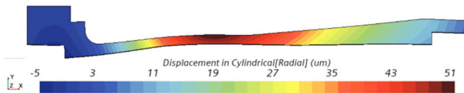
Fig. 3.9 Radial displacements of the optimized solution on a cavity section. Taken from [98]
