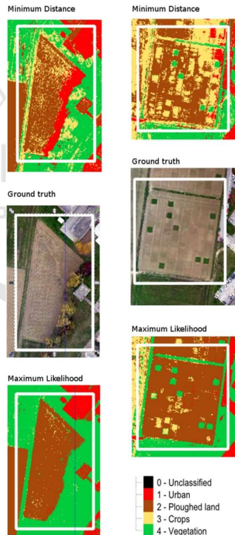
Figure 7: Comparison between classifications obtained two Minimum distance and Maximum likelihood algorithms.
