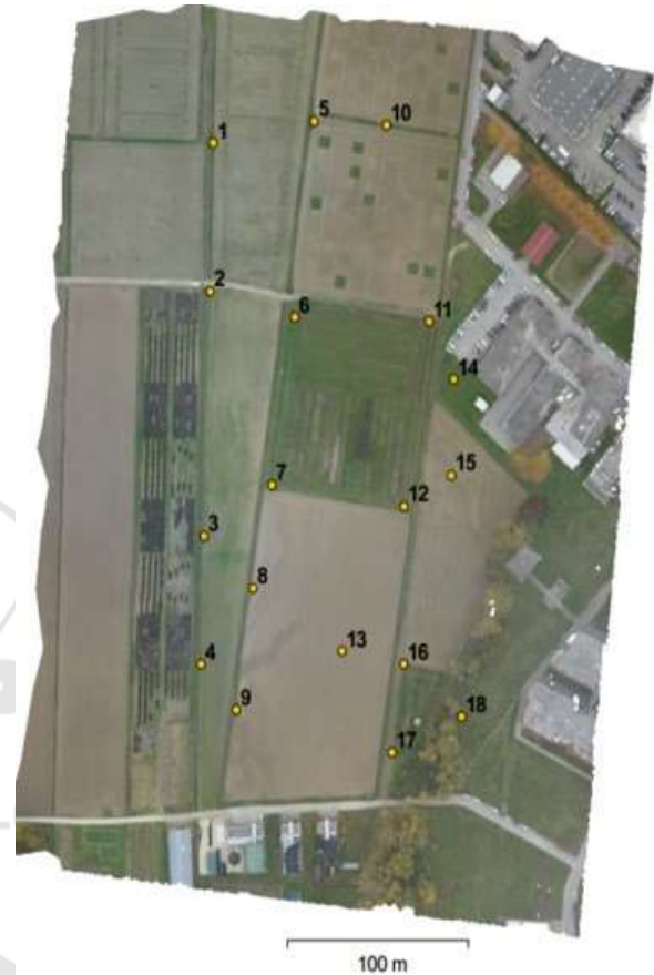
Figure 4: Position of the GCP in the testing area.
