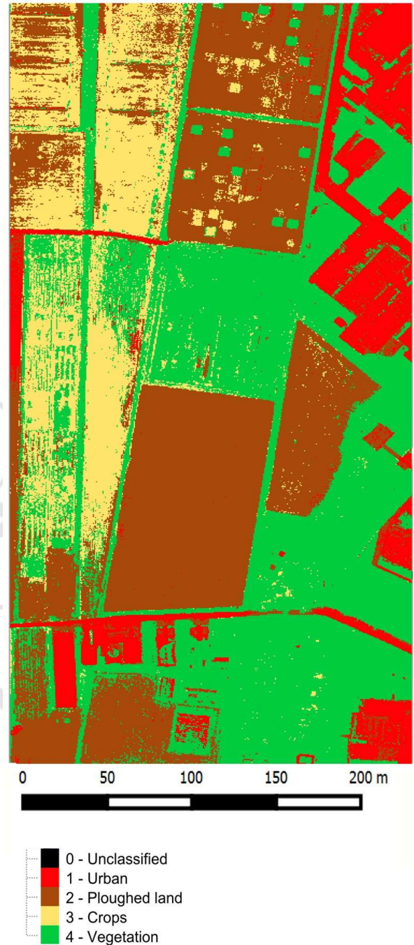
Figure 6: Classification with Maximum likelihood algorithm.
