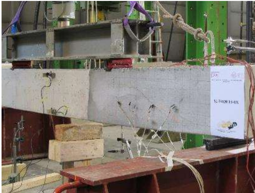
Figure 3-16 Crack pattern of beam for beam S1-FRCM-F3-UN for load P=150 kN
