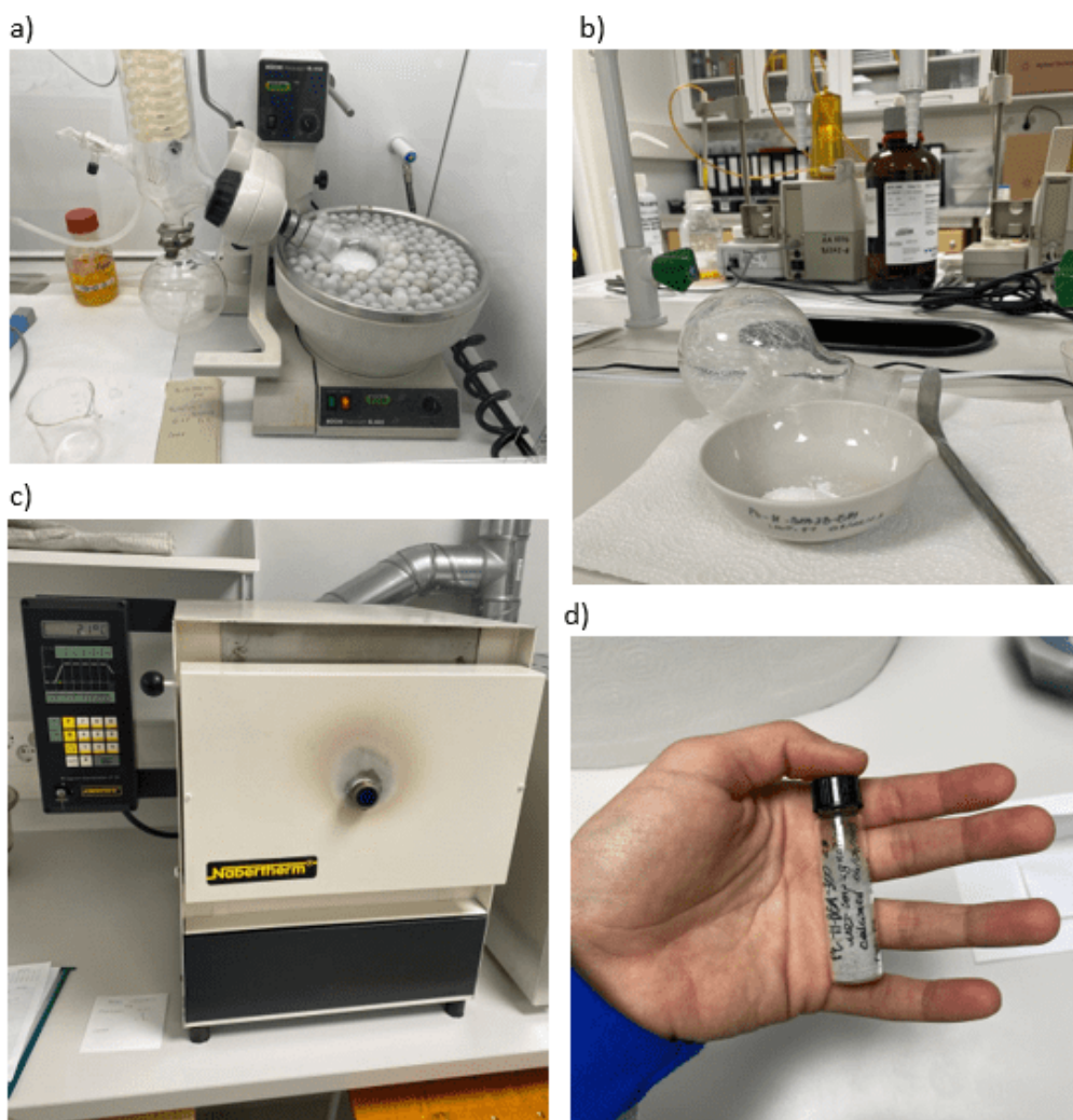
Figure 5.2: The most significant phases of the EIM method: a) the zeolite-platinum solution is rotated and solvent evaporated in a rotovaporator, b) the white powder, scratched from the flask walls, is transferred into a crucible, c) after drying, calcination is performed in a muffle oven, d) the Pt-modified catalyst, in the form of a greyish powder, is stored in a vial.
