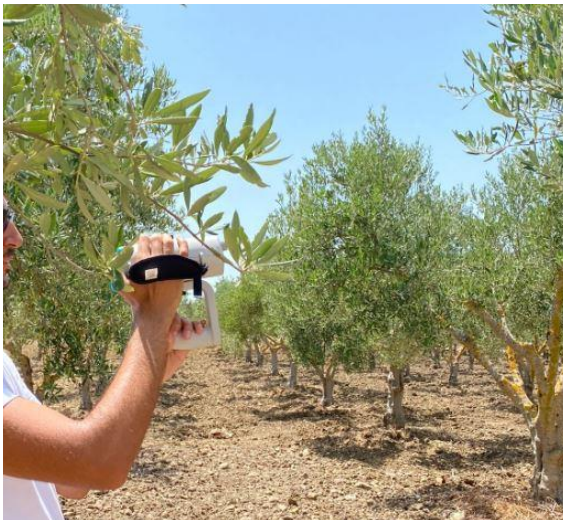
Figure 18. Proximal data acquisition with the hyperspectral sensor.
