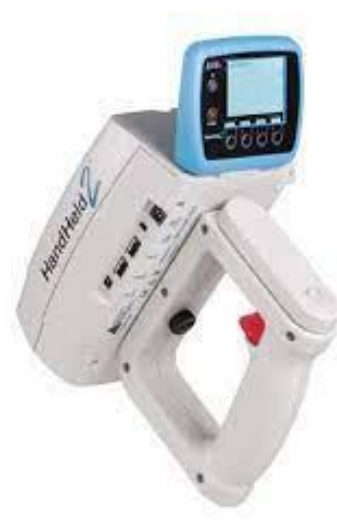
Figure 18. Proximal data acquisition with the hyperspectral sensor.
