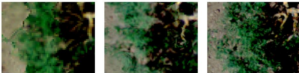
Figure 52. Different geometric resolutions from the flights 3c, 3b and 3a.
