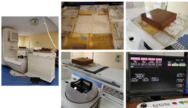
Fig. 10 On the left the Siemens Primus clinical linear accelerator (Siemens Medical Systems, Concord, CA, USA), from the Medical Physics and Radiation Oncology Department, ARNAS-Civico Hospital (Palermo). On the right the irradiation set up, from the plates positioning - between the slabs - until the setting of the dosimetric parameters.
