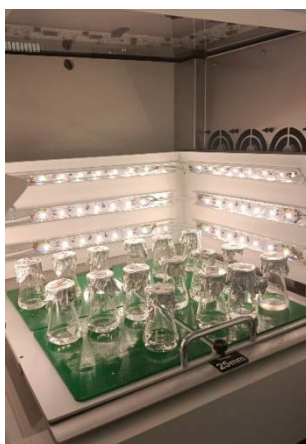
Figure 21. Photography of the apparatus for biological synthesis of ZnO with light in the incubator including an adapted LED system.
