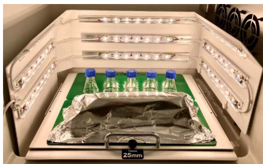
Figure 22. Setup of white light irradiation experiments in the incubator including an adapted LED system 86
