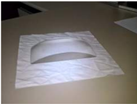
Figure 2.70: Picture of the planoconvex lens used as Cherenkov radiator for the beam tests.
