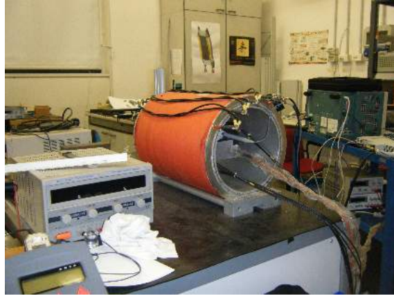
Figure 2.22: A picture of the setup used for the tests of the R11265 MaPMT in magnetic field.
