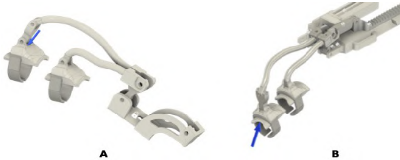
Figure 8.8: Models of the index module used for FEM analyses. In all the subfigures the finger's support is made with ABS while the ring is composed by soft plastic material. A CAD model of the old index finger module solution, where the mechanism and the linear actuator's support are made in ABS. B is showing the CAD models of the new index finger module solution, where the finger mechanism and the differential mechanism support are made in aluminum. Blue arrows represent the applied forces while the area signed with a white padlock indicates the constrained parts.
