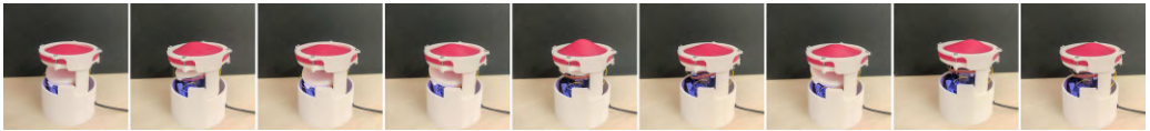
Figure 10.7: From left to right, the nine discrete positions reached by the haptic device.
