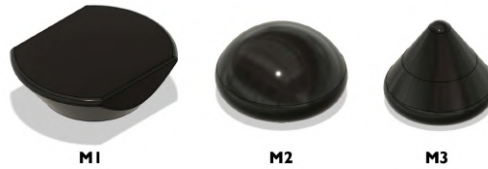
Figure 9.2: Modules of the new HapticPalm. M1 the plane-shaped module, M2 and M3 the spherical modules.
