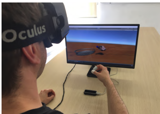
Figure 5.1: The user wears a head mounted display and interacts with a virtual object exploiting Self Contact. The virtual fingers are in contact with the virtual object when the user's fingertips are in contact with each other. The hand is tracked through a Leap Motion placed on the table. The virtual scene is repeated on the monitor for explanatory purposes only.
