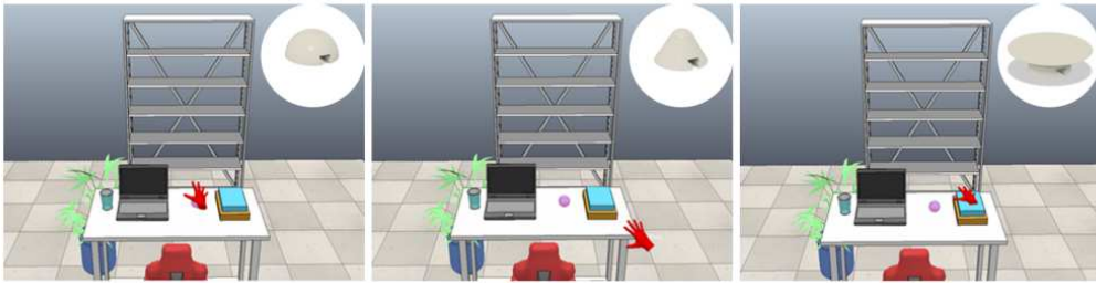
Figure 7.14: The testing virtual scenario is composed of a rack and a plant in vase in background and a office station in the foreground. The interaction is provided by the red hand avatar of and the objects in foreground are chosen to use all modules: paperweight for H1 module, cover of book and surface of desk for H3 module and desk, laptop and book peaks for H2 module.
